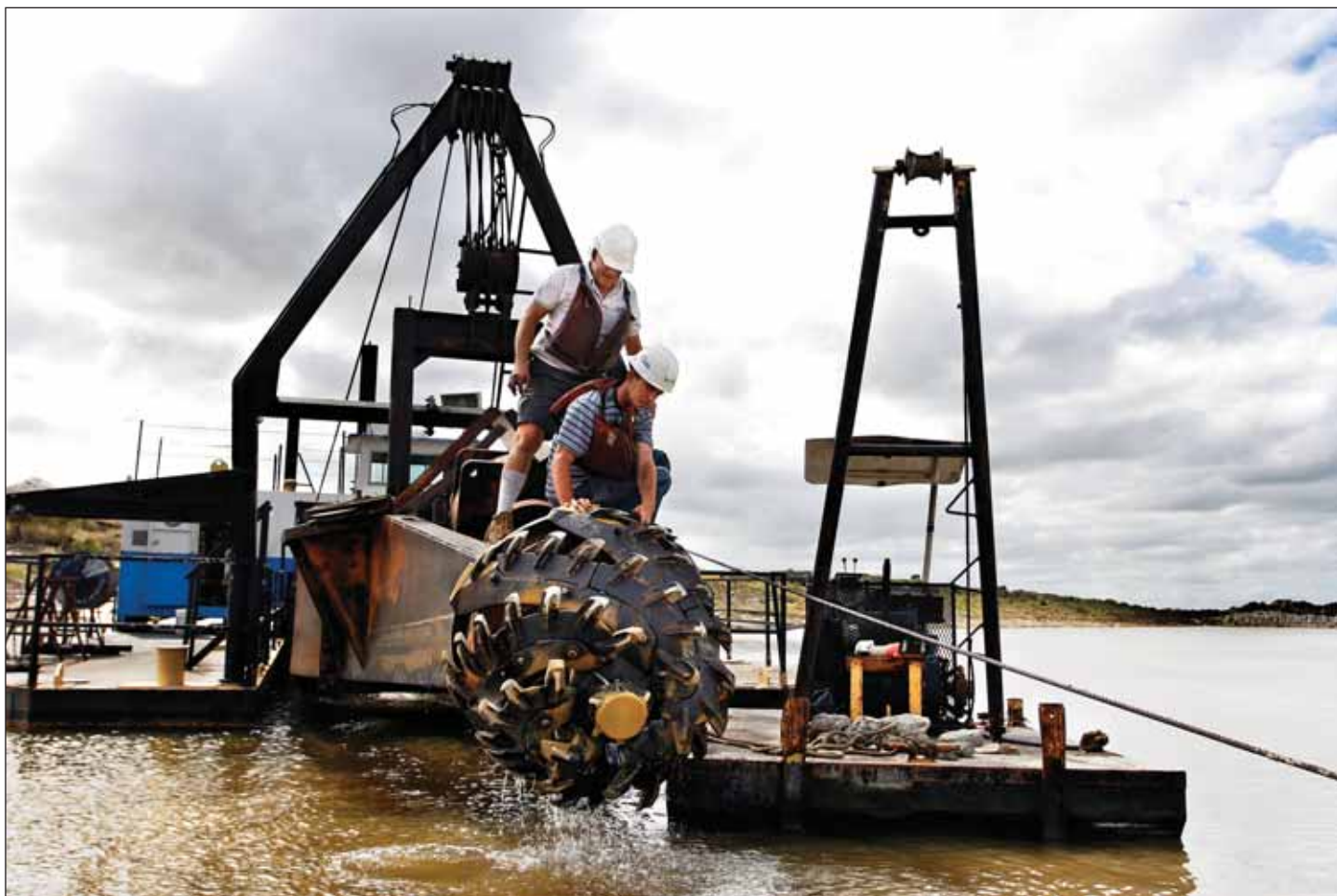
Pete Summerlin and Jimmy Thomas climb out to the end of the dredge to remove a large rock from the teeth of cutter head at the Ranch Road Lake Sandmine. Photos: Tom McCarthy Jr.
